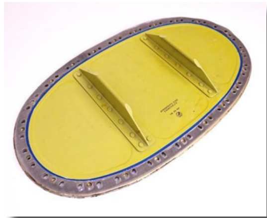
MD-80 fuel resistant conductive gasket.
