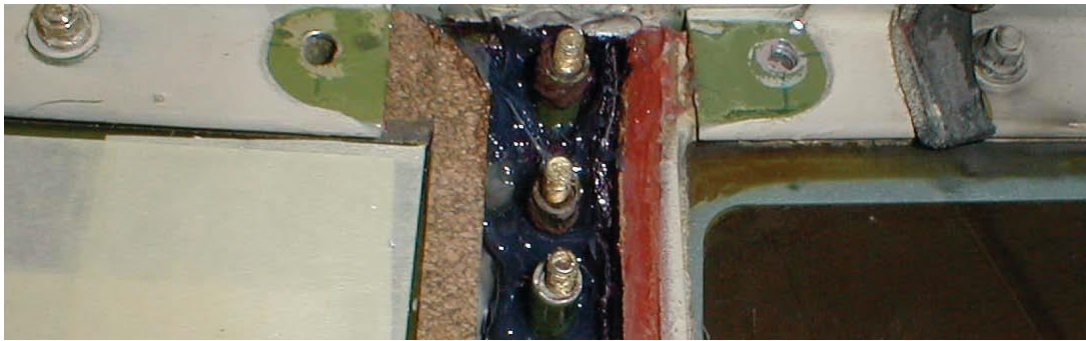
C130 Interior Window Installation
