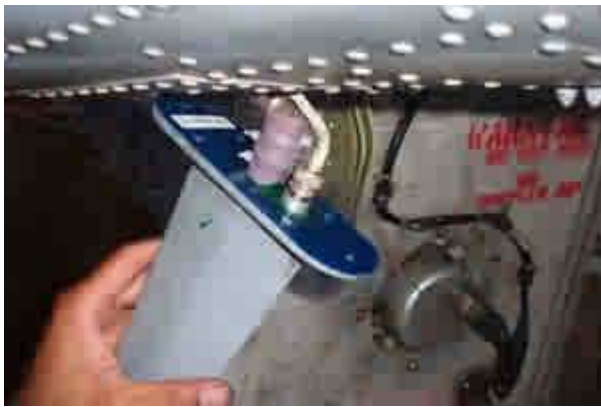
U.S. Navy technicians apply an Av-DEC sealant system to the antenna interface of an H-60 Seahawk helicopter. Photo courtesy of Av-DEC.
