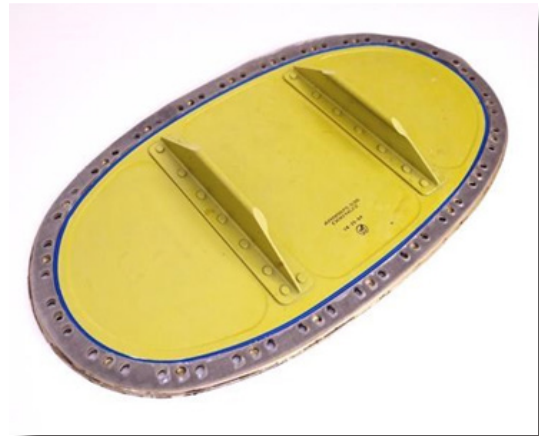
MD-80 fuel resistant conductive gasket.
