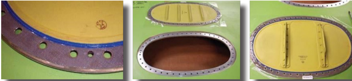
MD-80 fuel resistant conductive gasket.
