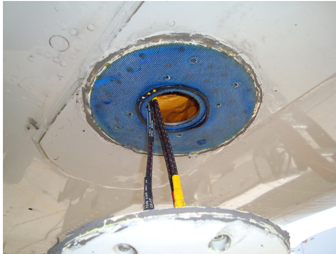
HI-TAK® Polyurethane Conductive Gasket installed on TCAS antenna
