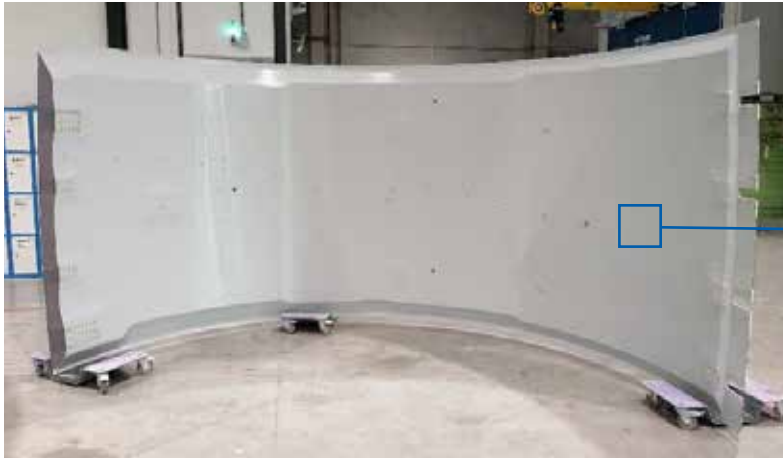
777 fan cowl door sprayed with SpraySeal®.
