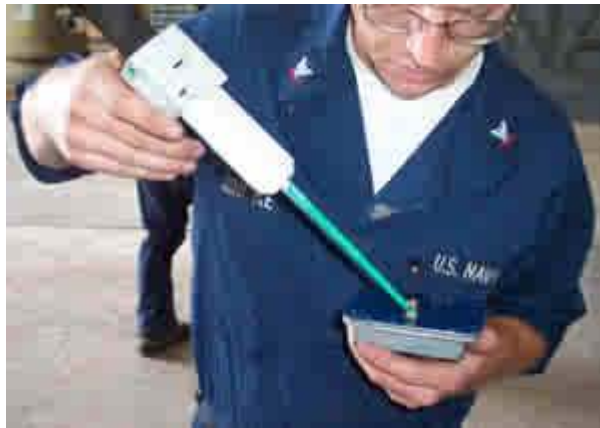
U.S. Navy technicians apply an Av-DEC sealant system to the antenna interface of an H-60 Seahawk helicopter. Photo courtesy of Av-DEC.
